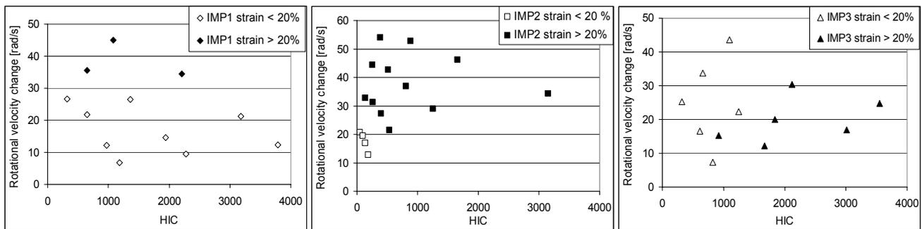
Fig. 2 - Results from the three different impacts. To the left impact 1, in the middle impact 2, and to the right impact 3. The levels on the axes are computed levels in the FE Model of the HIII head. Filled points represent injurious strain levels in the brain.
