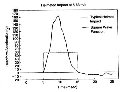
FIGURE 14.8. Typical helmeted head form acceleration trace.
