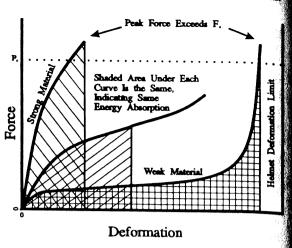
FIGURE 14.6. Effect of padding strength when the same energy is absorbed.
