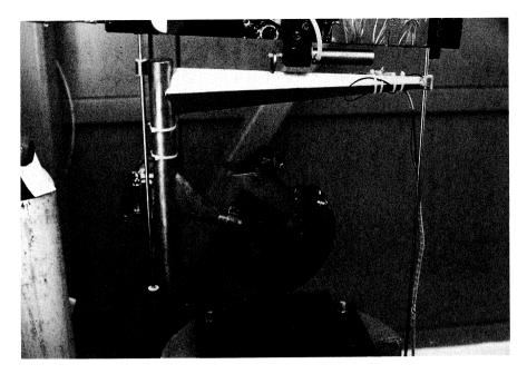
FIGURE 14.7. Typical helmet-impact vertical-drop test setup.
