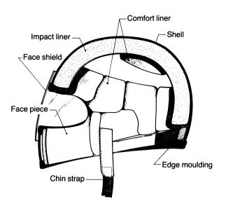
FIGURE 14.1. Cross section of a typical motorcycle helmet.
