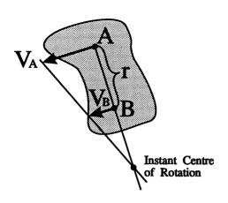
FIGURE 14.3. Free body in motion.
