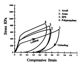
FIGURE 14.5. Stress-strain of padding.
