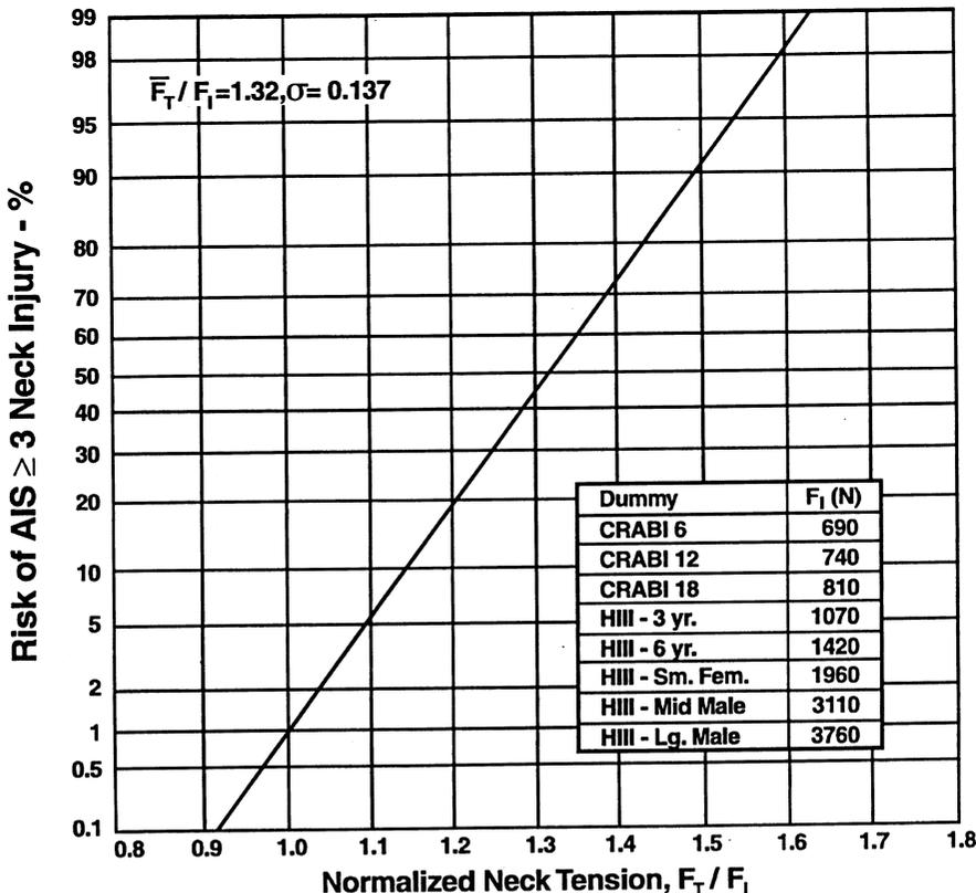
FIGURE 5.4. Risk of AIS ≥ 3 neck injury as a function of normalized neck tension for the child restraint airbag interaction (CRABI) and Hybrid III dummy families. Minimum muscle tone.
