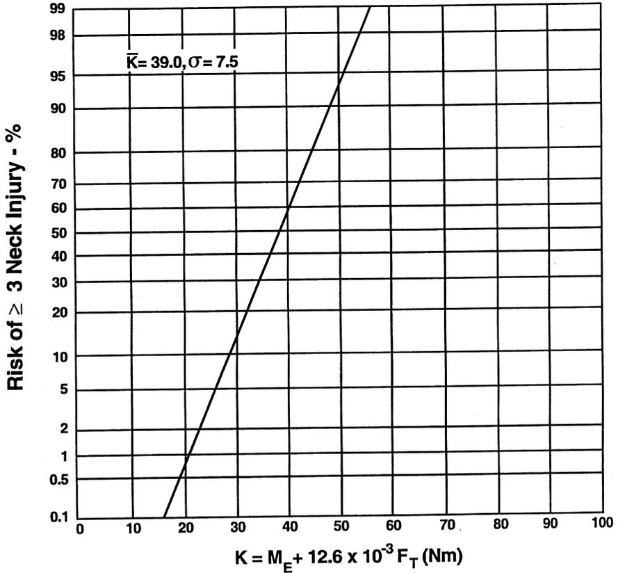
FIGURE 5.6. Risk of AIS  $\geq 3$  neck injury as a function of combined neck extension moment taken with respect to the occipital condyles and neck tension for the Hybrid III 3-year-old dummy. Minimum muscle tone.
