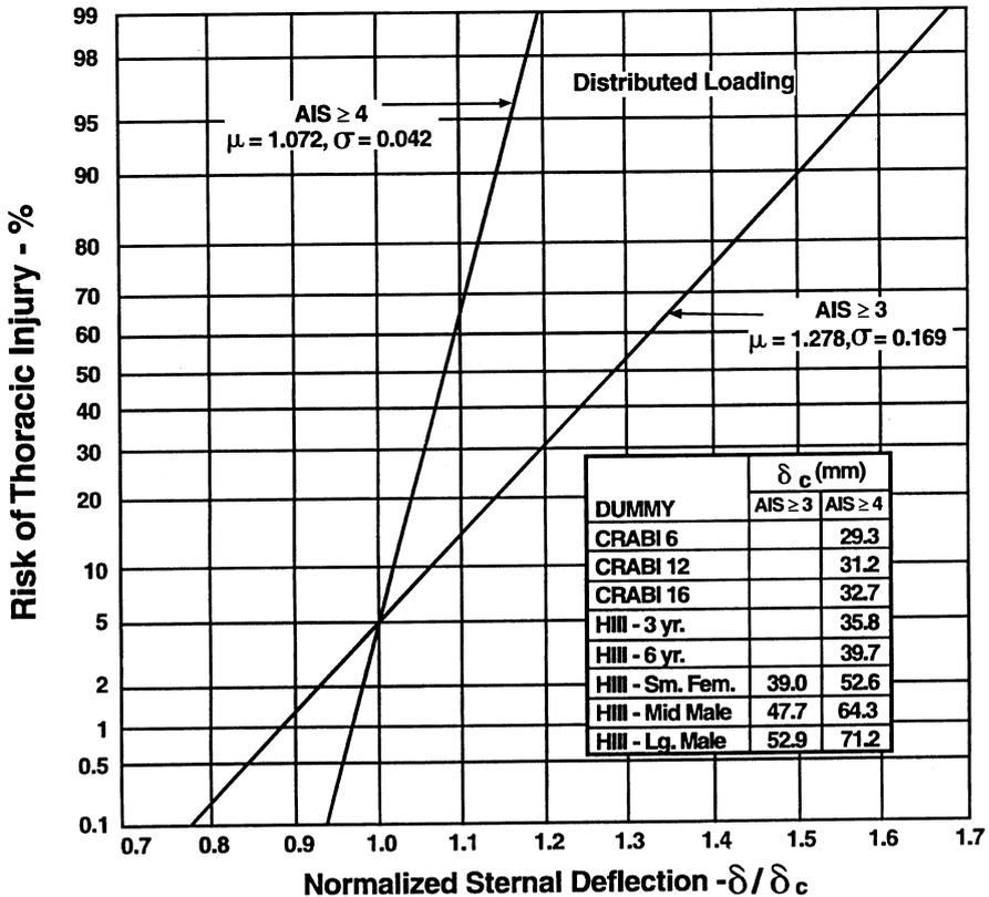
FIGURE 5.8. Risk of AIS  $\geq 3$  and AIS  $\geq 4$  thoracic injuries for CRABI and Hybrid III dummy families as a function of normalized sternal deflection due to distributed anterior thoracic impacts.
