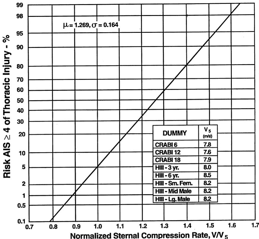
FIGURE 5.10. Risk of AIS  $\geq 4$  thoracic injury for CRABI and Hybrid III dummy families as function of normalized sternal deflection rate due to distributed anterior thoracic impacts.
