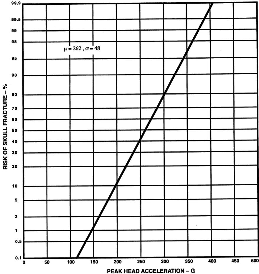
FIGURE 5.3. Risk of skull fracture as a function of peak resultant acceleration of the center of gravity of the head for forehead impacts.
