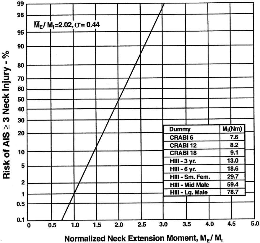
FIGURE 5.5. Risk of AIS ≥3 neck injury as a function of normalized neck extension moment for the CRABI and Hybrid III dummy families. Minimum muscle tone.
