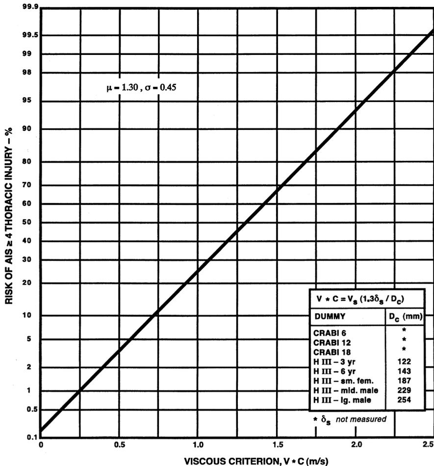
FIGURE 5.11. Risk of AIS  $\geq 4$  thoracic injury for adult dummies as a function of peak viscous criterion for distributed anterior thoracic impacts.
