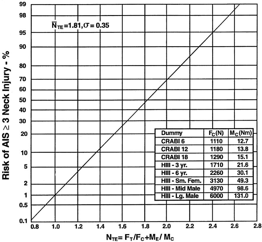
FIGURE 5.7. Risk of AIS ≥3 neck injury as a function of combined normalized neck extension moment taken with respect to the occipital condyles and neck
