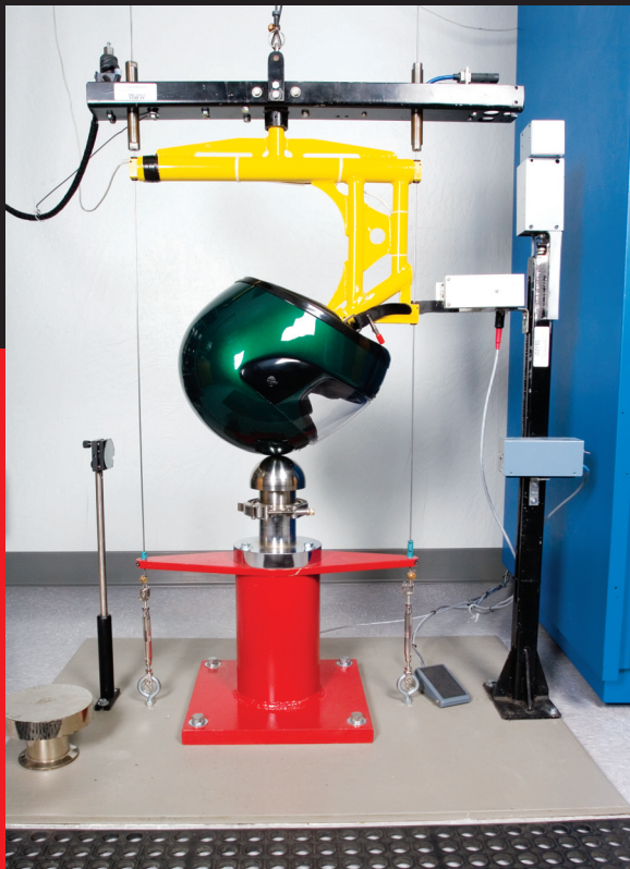
The SNELL Memorial Foundation uses many tests in order to certify a helmet with a SNELL M2010 designation. The photos you see here were taken inside the testing facility and show some of the tests and the aspects involved. The SNELL test stand, above, measures a helmet's ability to withstand impact forces.
