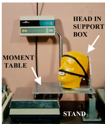
Figure 1. Manikin head in XR-50 Mass Properties Instrument being measured for CGx.
